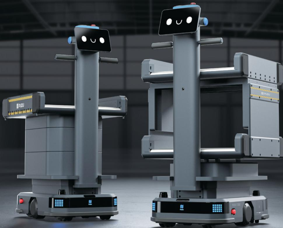
The T300 Conveyor is equipped with a self-powered roller system, enabling seamless integration with automated conveyor lines and other material handling equipment. It facilitates efficient material transfer and transportation between different stations.
